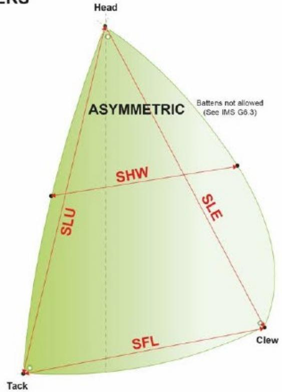
G6.1 half width of any spinnaker shall be 75% or more of the foot length. If not, the sail shall be measured as a headsail
