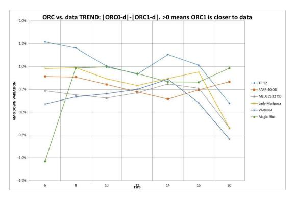
The plots are showing the movement of the VPP speeds related to the recorded speeds in %. If the value is positive it means that the gap is reduced, if the value is negative the gap is increased. As can be seen (apart some uncontriled movements at 6kts and a boat – KER 56 VARUNA – that has some unreliable data according to his designer) the modifications introduced are working in the expected direction by reducing the gap between the observed data and the VPP.
