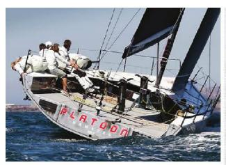
When maximum beam runs all the way aft (above) then 'diagonal heeling' (top) is the inevitable result. An increasing challenge for the creators of grand prix racers like this TP52. Imoca and open class designers have wrestled with this phenomenon for years
