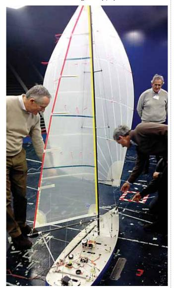
Chair Alessandro Nazareth (left) and other ITC members joined North Sails Italy in a recent continuation of sail tests in the wind tunnel at Milan Polytechnic. The goal is to refine calibration with a parallel study using OpenFOAM software at the Wolfson Unit
